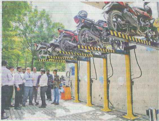
Hydraulic two-wheeler parking facility at Meenambakkam Metro Rail station
