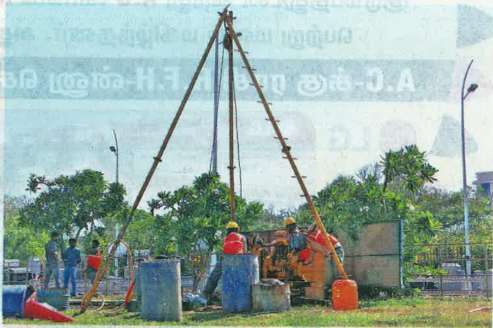
METRO MARINA Chennai Metro Rail Limited (CMRL) workers involved in soil tests and geo-technical investigations on the Marina beach near Gandhi statue on Saturday
