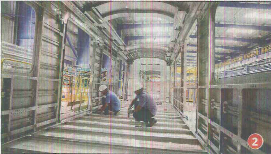
THE STOPS: 1. Stainless steel outer shell arrives at the car body shell shop 2. Structure of the train-side and end wall is welded with the roof and under-frame to make the body of the coach 3. Electrical components including the traction system, cables and wheelset are installed under the body of the coach in the fitting shop 4. The mask of the train operator cabin is fitted to steel frame 5. After a series of tests, the bogies are sent for integration before trial runs
