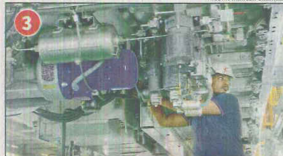
THE STOPS: 1. Stainless steel outer shell arrives at the car body shell shop 2. Structure of the train-side and end wall is welded with the roof and under-frame to make the body of the coach 3. Electrical components including the traction system, cables and wheelset are installed under the body of the coach in the fitting shop 4. The mask of the train operator cabin is fitted to steel frame 5. After a series of tests, the bogies are sent for integration before trial runs
