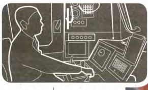
he operator will monitor passengers entering and exiting a train through screens installed in his cabin, control doors and perform other related functions. Each coach will be connected by intercom for emergency communication between passengers and the driver
