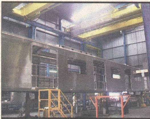
A shell of the metro rail coach being manufactured at La Pa in Brazil
